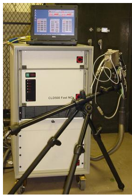
Figure 3.3 Fast NO analyzer (CLD500) provided by Cambustion [66].
